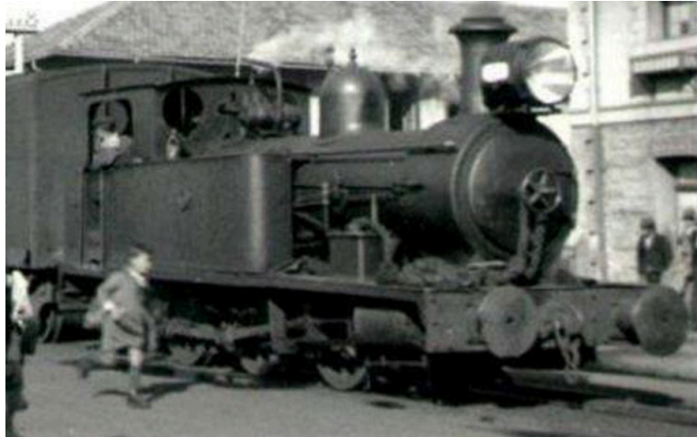
One of these engines on a passenger train along the main street in Puchoco-Schwager. A turbo-generator has been added in front of the safety valves to power the large electric headlight.
