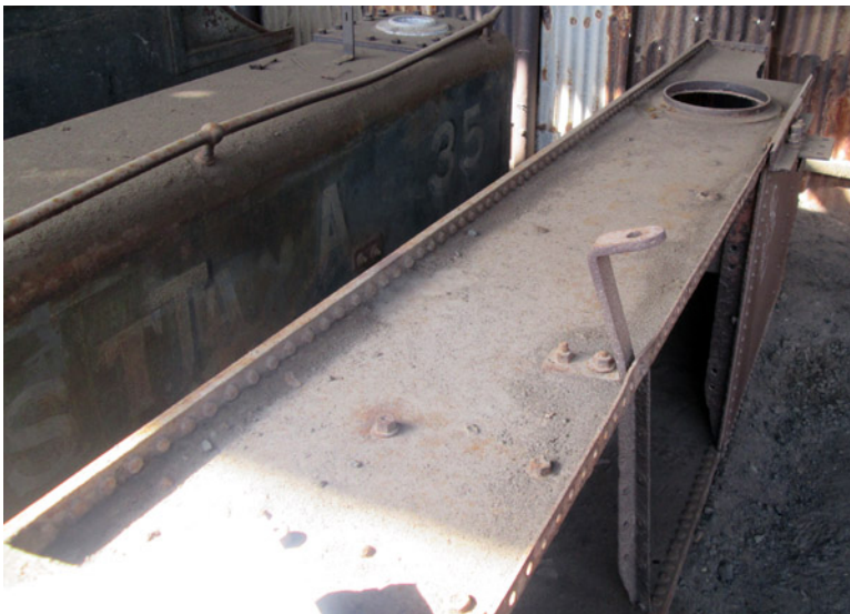
RH Tank 402cm length, 46cm thick, 96cm tall, No cutout It bears the no. 21, and had carried a big nameplate with a worksplate above it.
