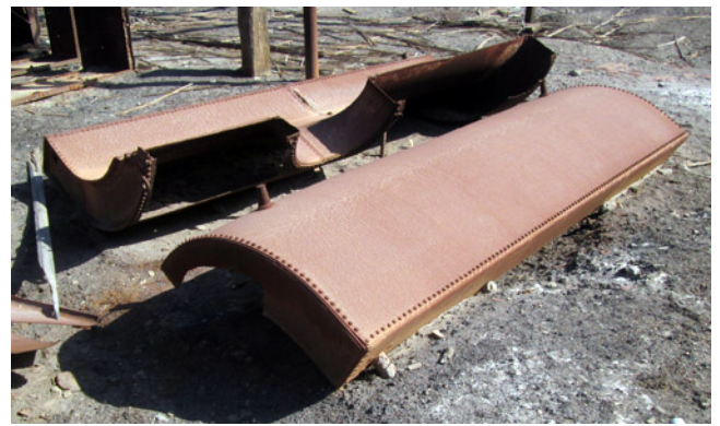
Saddle tank 320cm length, 128cm distance of dome c/l from one end, 98cm top to bottom. This might be from one of the FC de Agua Santa 2-4-2STTs by Baldwin.
