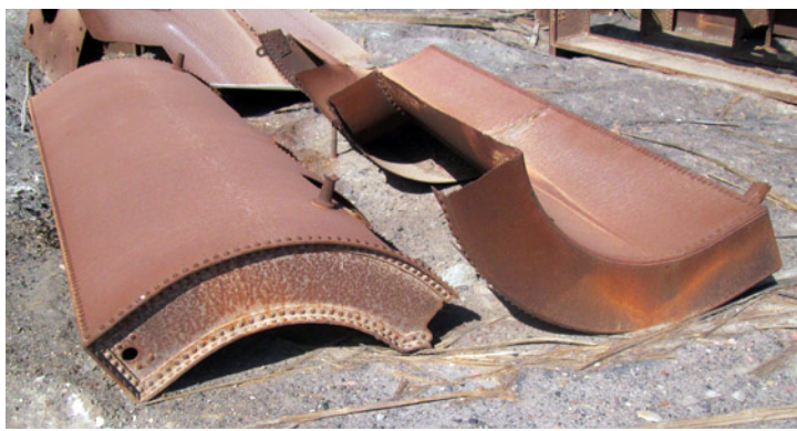
Saddle tank 320cm length, 128cm distance of dome c/l from one end, 98cm top to bottom. This might be from one of the FC de Agua Santa 2-4-2STTs by Baldwin.
