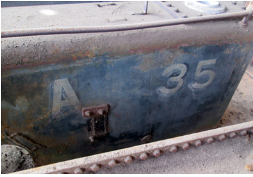
LH Tank 340cm length, 100cm height, 50-54cm thick, inside face curves to follow boiler, 182 x 37cm cutout
