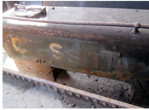
LH Tank 340cm length, 100cm height, 50-54cm thick, inside face curves to follow boiler, 182 x 37cm cutout
