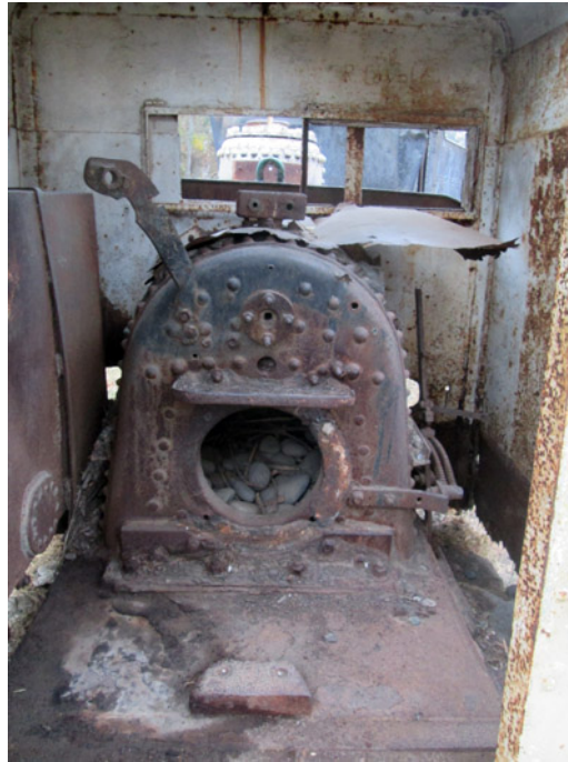
The cab of the surviving loco at Balneario Cachapoal. The oil tank filling the left side demonstrates why there are no windows on that side.
