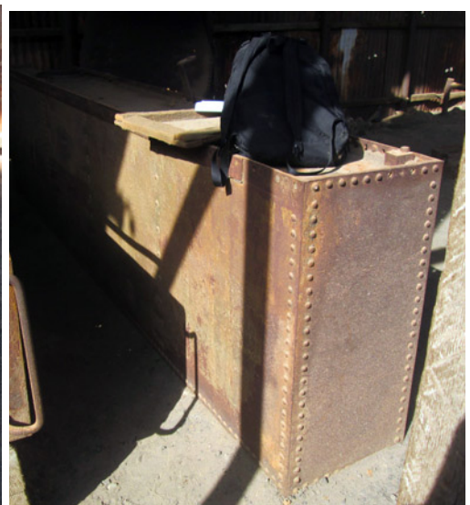
RH Tank 402cm length, 46cm thick, 96cm tall, No cutout It bears the no. 21, and had carried a big nameplate with a worksplate above it.
