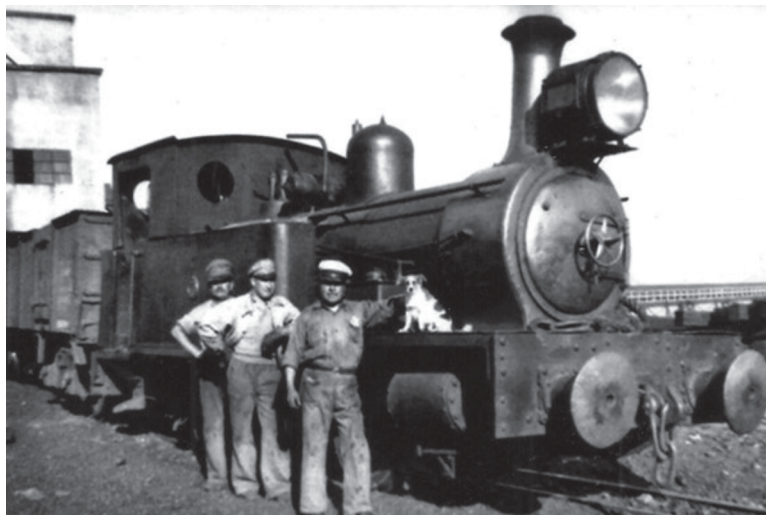
One of these three locos in use, seemingly with a slightly taller chimney than in the photo above. The engine is standing on mixed gauge track and the sheer size of the bogie coal wagon behind it suggests that it may have been a broad gauge vehicle belonging either to the EFE or to the FC de Arauco . This loco has a deeper buffer-beam and therefore a higher and stepped running plate when compared with those illustrated above. Whether this was as built or as modified later is currently unknown.
