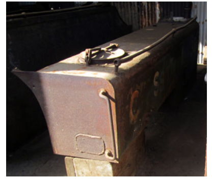
LH Tank 340cm length, 100cm height, 50-54cm thick, inside face curves to follow boiler, 182 x 37cm cutout
