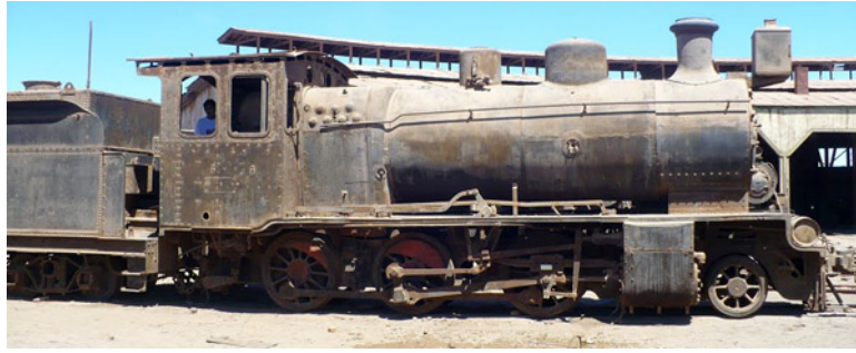
3223 as surviving at Baquedano. The loco has gained a bogie tender in place of its original six-wheeled one, and this has had its sides raised either before or when the oil tank was dropped into the bunker.
