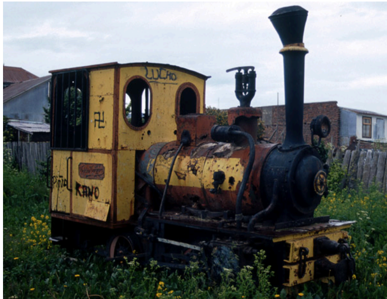
The same loco, renamed ' VALDES VERGARA ', lying forlornly in a yard behind the town museum in 2000. The safety valves are clearly an in-service modification.
