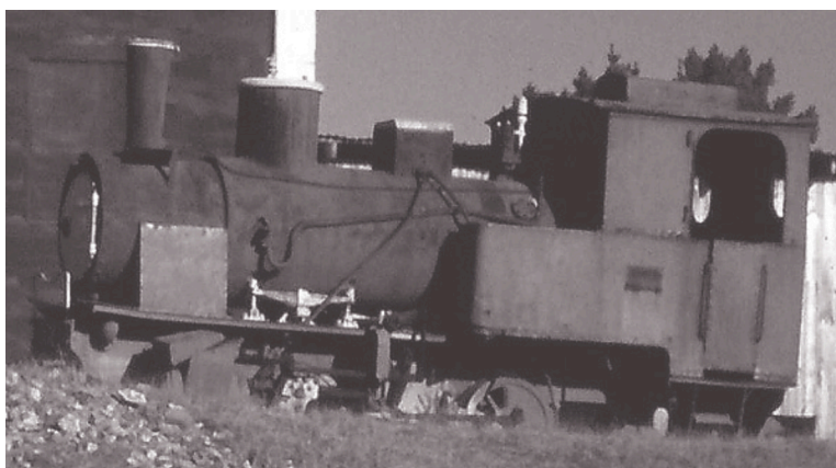
This appears to be identical to the two Jung 0-4-0WTs built for the paper mill at Constitución to the gauge of 900mm. Further work is needed to clarify this.
