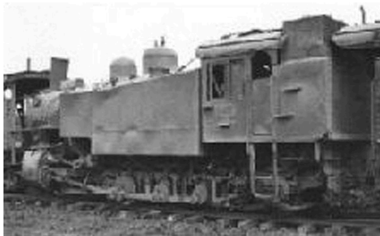
Photo by David Ibbotson from 1955, showing tank extension, and modified cab and bunker.
