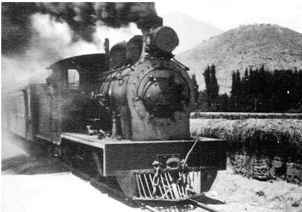
One of these engines, with an added sand-dome and electric headlight, possibly along the San Clemente branch south-east of Talca.
