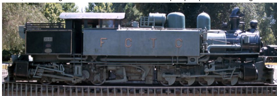
MCC's own pic of no. 9 ( EFE no. 3349) taken at Quinta Normal museum. Note the altered cab roof, added sand dome, and extra air tank; also the disappearance
