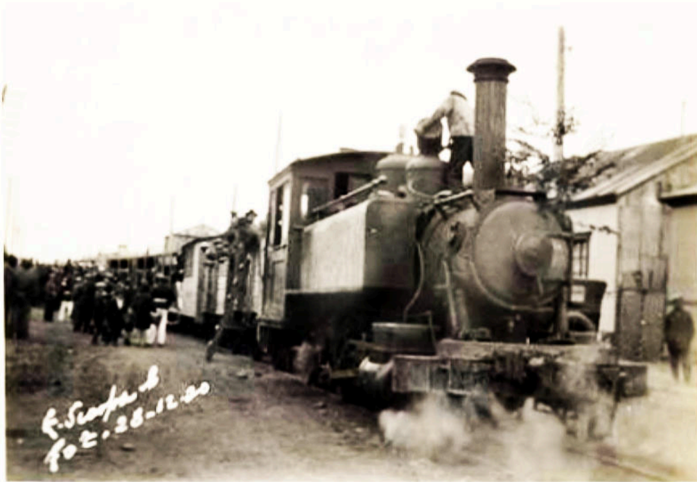
One of the two larger Baldwin 0-4-2Ts on a train in December 1920. Photo provided by courtesy of Sr. Pablo Moraga.
