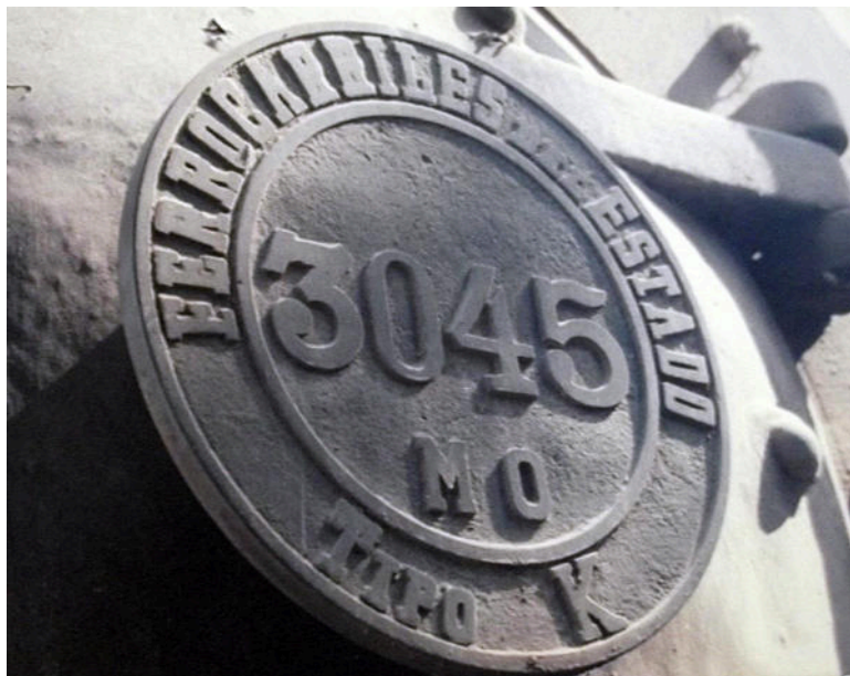
The smokebox numberplate of no. 3045 , with the inscription 'MO' indicating that the engine had been under the supervision of Maestranza Ovalle.
