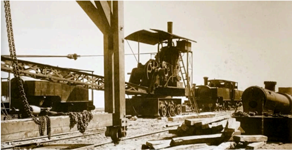
Three 'Huxley' class Kerr Stuart 0-4-2Ts and a slightly strange six-wheeled mobile crane,
