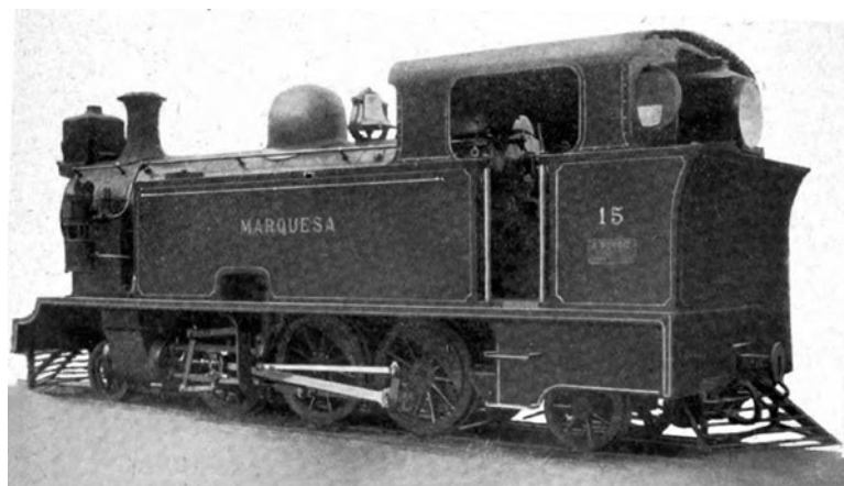
Borsig publicity photo. The steel valances behind the rear steps were later removed, presumably to improve access to the rear trucks.
