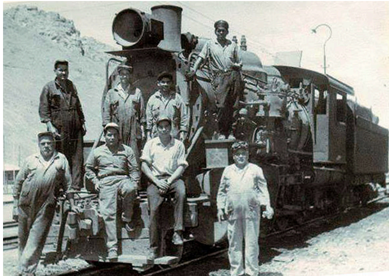
This is one of several photos showing one of the 2-8-0s at Barquito where it was probably located as a switcher/shunter. Note the front footstep fitted in place of the original pilot/cow-catcher.
