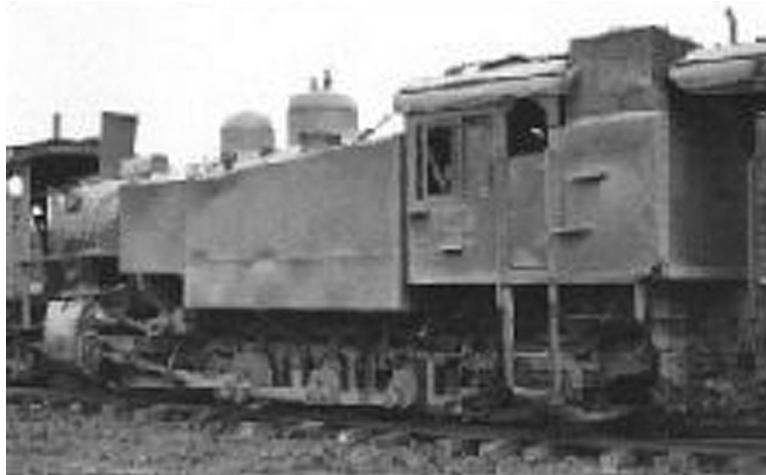
Photo by David Ibbotson from 1955, showing tank extension, and modified cab and bunker.
