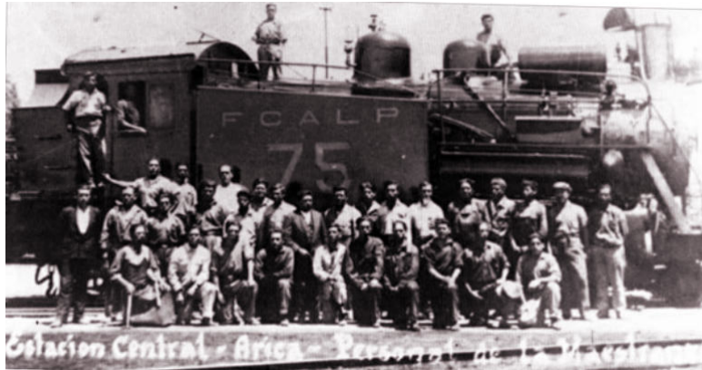
The same loco as later numbered 75 , and with additional air tank or counter-pressure brake header tank on boiler top, handrail along running plate and tanks, and with full height oil tank in bunker.
