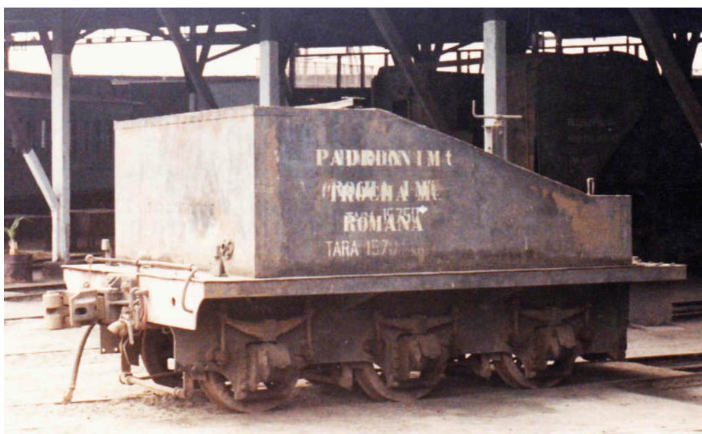
The remains of a 6-wheeled metre gauge tender being used as a tank wagon at Maestranza El Colorado in Iquique. It's origin is currently unknown.
