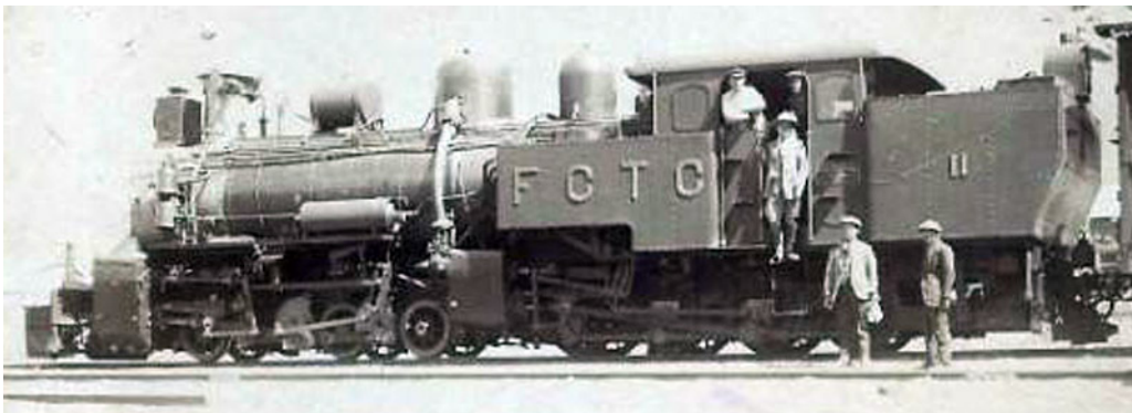
No. 11, on the other hand has a short 'lower step' to its new tanks, as its cab entrance was further forward. The drum tank mounted above the boiler was a header tank for the counter-pressure brake.
