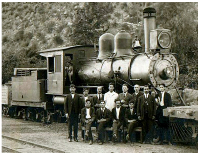
The photo here seems to show one of these two engines on the Elqui line at an unknown date, albeit with a replacement cab, bell and chimney.
