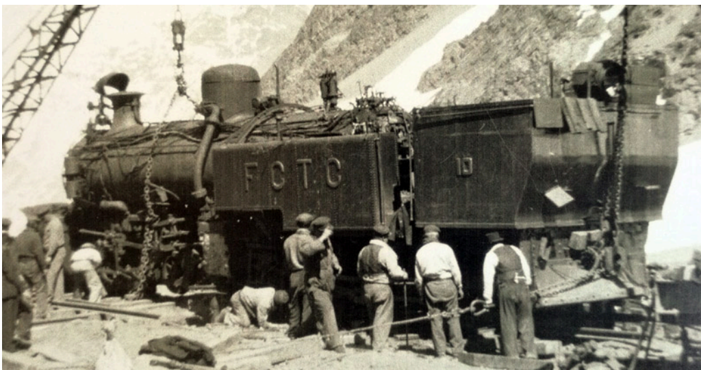
No. 10, seen being recovered after a derailment in 1944, and with replacement tanks, having a long 'lower step' and a cab entrance immediately in front of the bunker.
