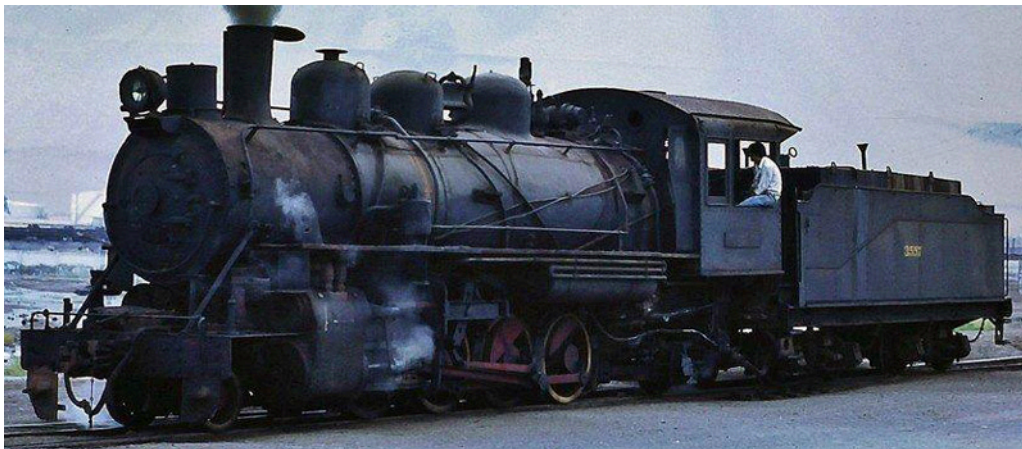
Tipo W no.3557 at Iquique at an unknown date, seemingly still bearing its name-plate. Note the slightly larger tender than in the first picture above, and that the rear sand dome has been moved forward and is now just behind the front sand dome, as also in the second image of no. 3511 above..
