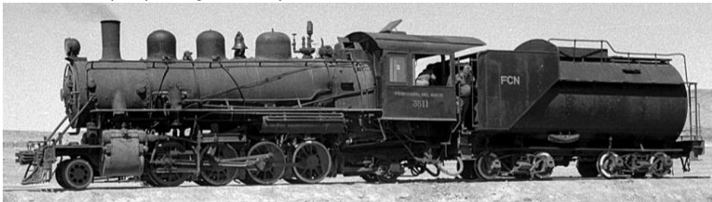
No. 3511 seen rather later, now with Vanderbilt tender, air pump just behind the cylinders, the second sand dome moved forward, and the turbo shifted back from before the chimney to in front of the cab.
