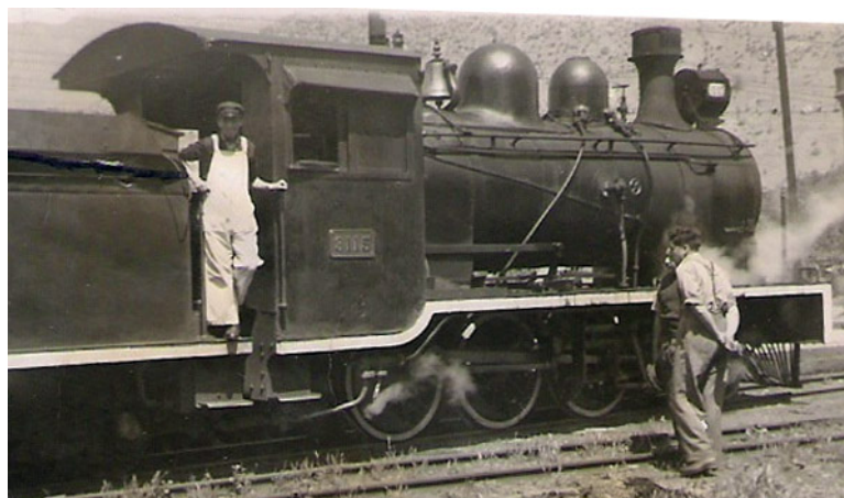
Tipo T no. 3115 . Note again that the air pump has been moved to the left side, possibly to improve sightlines for the drivers.
