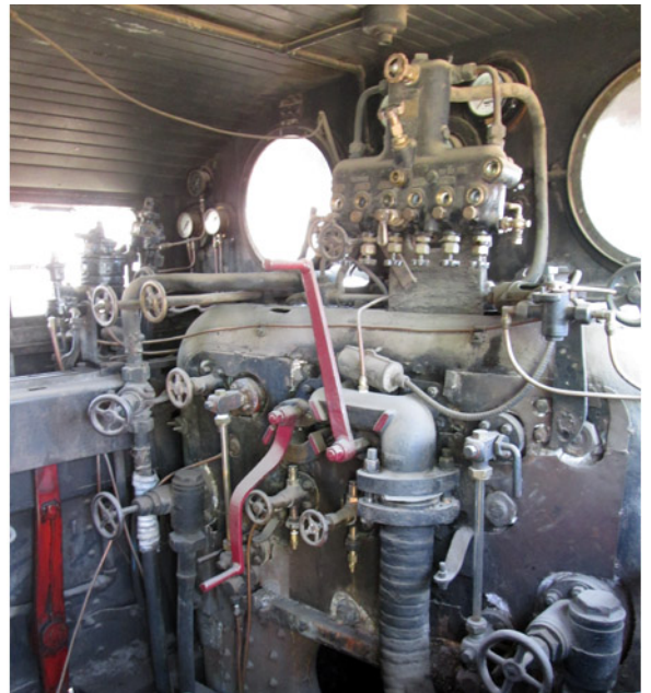
Views within the cab of no. 8 / 3348 at Los Andes shed in 2016. The left hand photo shows the reverser handles and wheel – separately controlling the rack and adhesion cylinders. The right hand picture shows the two separate regulator handles – adhesion on the left and rack on the right – also the six-feed lubricator above and the extremely long gauge glasses in order to allow for a wide range of gradients.
