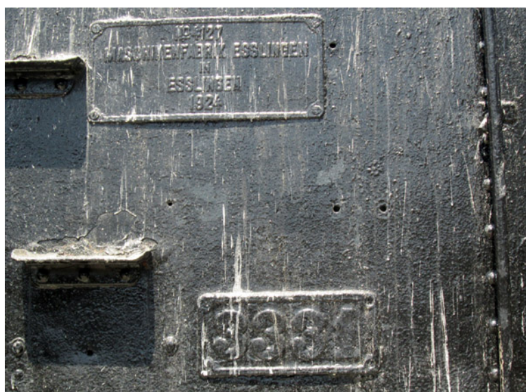
Tipo Uc no. 3315 (as evidenced by the worksplate number) as plinthed in Arica in 2019, but falsely bearing a number plate from Ua no. 3331 . A comparison of the boiler diameter and chimney height with that of a Ua loco in the next photo down, will illustrate that the Uc engines were slightly smaller. Ian Thomson has suggested that the loco is actually no. 3317 , but from what evidence is unknown.
