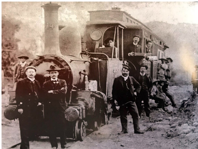
Neilson 2-4-0T no 2381 running as DOP no. 14. Noteworthy points are the
