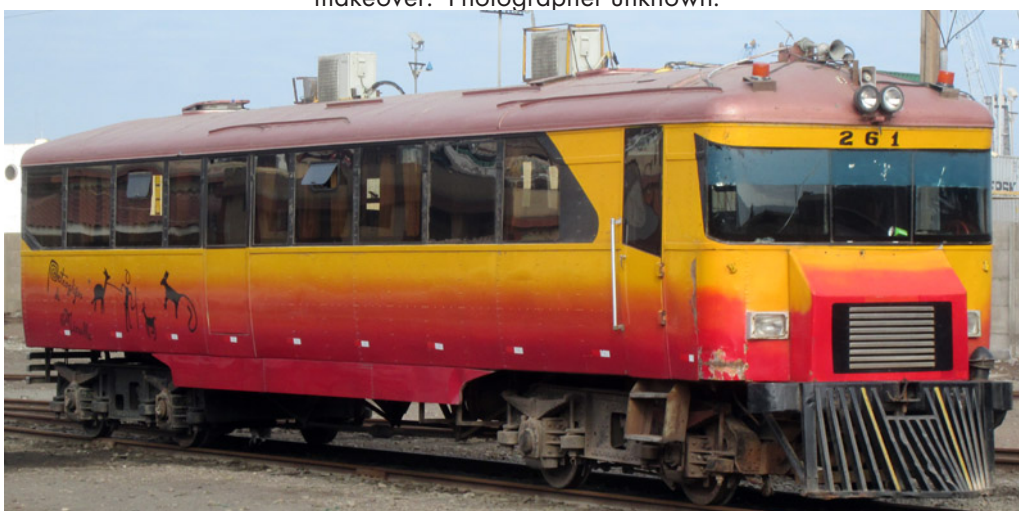
Railcar 261 in its present guise. Whilst the windows, paintwork and roof-mounted AC units suggest radical changes, it seems likely that the bogies, frame and basic body structure date right back to the vehicle's construction in 1936.
