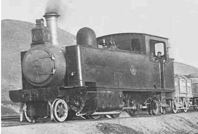
One of the 2-6-2Ts out on the pampa, still with its motion covers but now having extended side tanks and a longer smokebox. Note that these engines can be distinguished from the later locos built with long tanks by the trailing truck and rear bunker.
