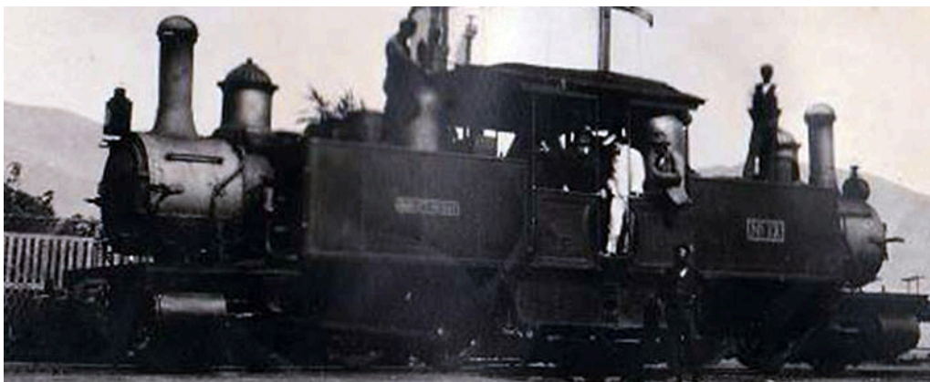
Two double Fairlies with numbers beginning with 1, though in neither case can the second digit be made out. Both seem to have straight-topped boilers, but the upper picture shows low cab sides which suggests that the engine is an earlier one than that in the second image which has a full wooden cab. The second one has full length fuel racks.
