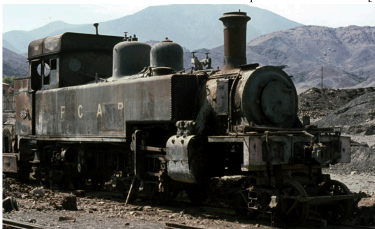
MCC's own photo of no. 30 , at Taltal in 1975, whilst supported on ambles bogies during re-gauging work.
