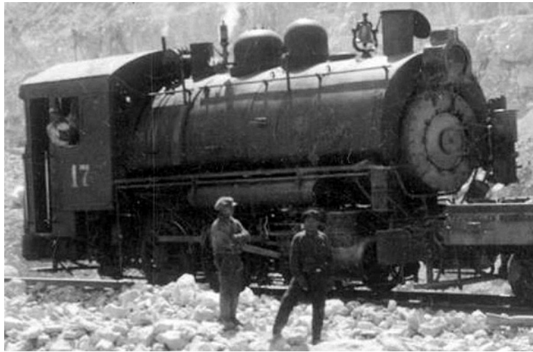
The above loco has a full-length saddle tank rather than one terminating at the front tube-plate. Thus far it has not been identified.
