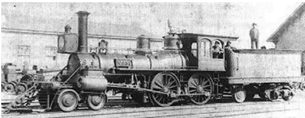
This photo shows Norris Bros. 4-4-0 no. 8 attached to a Hawthorn 2-4 wheel arrangement tender as supplied with loco no. 31 .
