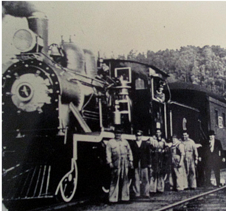
A Curanilahue tender loco on a train. Whilst the small steps in the running plate suggest that this was one of the two Borsig mogule, the smokebox looks different and has outside steam pipes. This needs further study.
