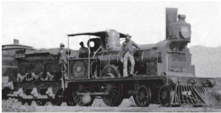
Whilst this is not a good image, it does seem to show one of the Hawthorn 0-4-2s as rebuilt to 4-4-0 configuration.
