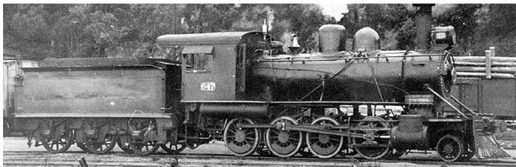
Tipo 69 no. 647 . The replacement boiler has been mounted higher than the original, probably because of a deeper firebox. The additional height of the smokebox above the saddle casting can be seen, also the shorter smokebox and round-topped firebox.
