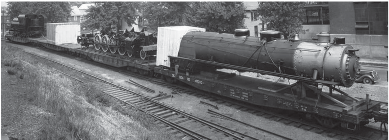
A tipo 110 leaves Baldwin's plant on four flats, bearing the tender, a crate of parts, the fully-erected chassis and the boiler.
