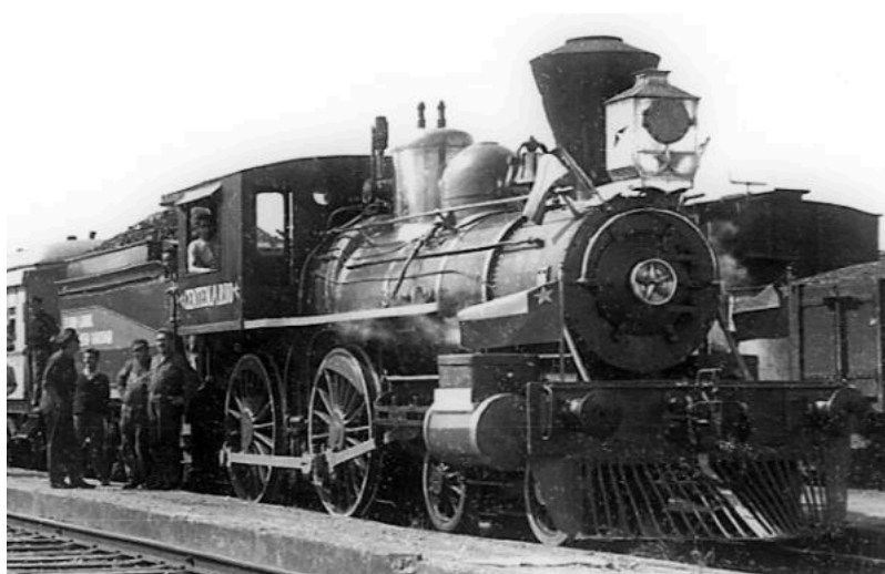
This is a tipo 20 , with added sand-dome and spark-arresting chimney, but more interestingly it has been painted up, probably for a fiesta Patria , with coloured tender (possibly in the national colours of white, red and blue) and the name ' CENTENARIO ' on the cab side.
