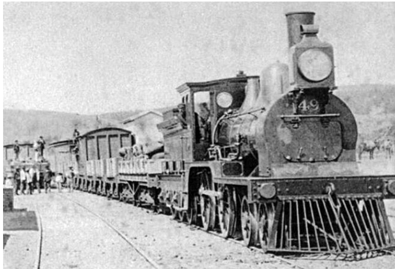
No. 49 , showing the original extremely small diameter buffers.
