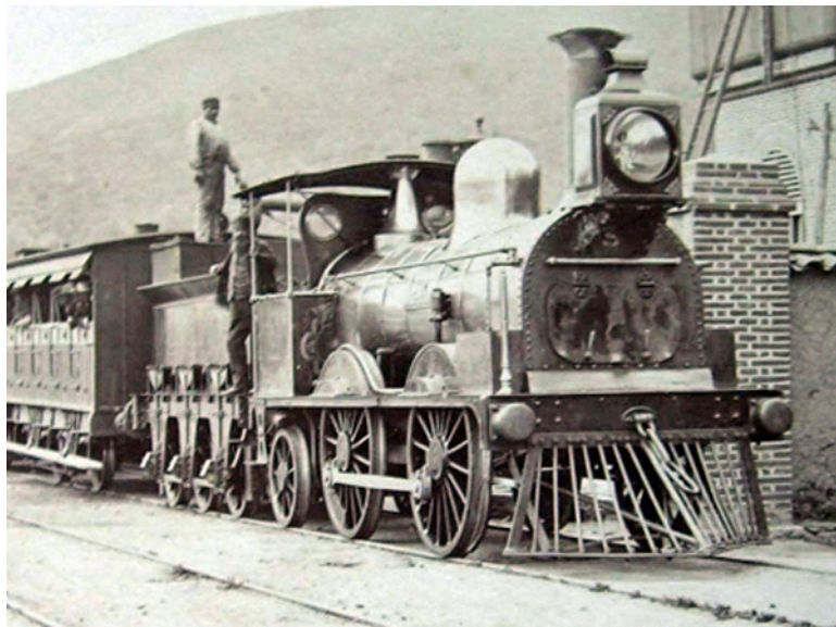
An intermediate condition, with a domed boiler, sandboxes and large oil lamp, but still with a capped chimney.
